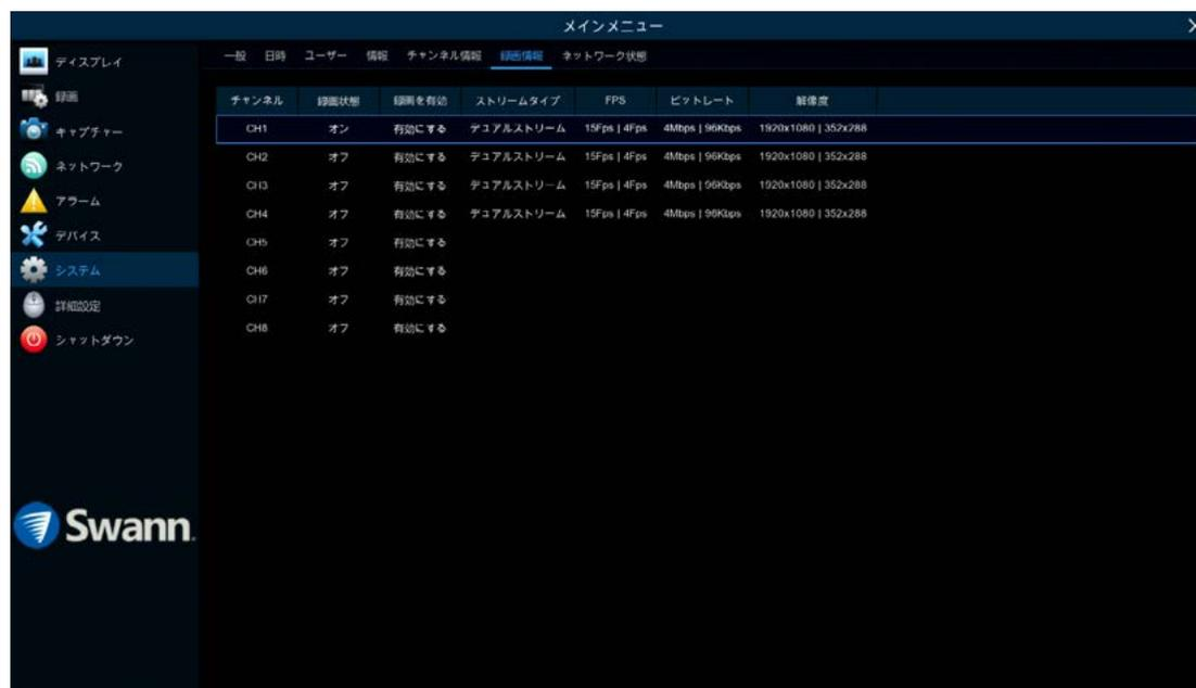
The screenshot shows a web interface for Swann system management. The '録画情報' (Recording Information) tab is selected, displaying a table of recording settings for eight channels (CH1 to CH8). The table columns include Channel, Recording Status, Recording Enabled, Stream Type, FPS, Bitrate, and Resolution. The Swann logo is visible in the bottom left corner of the interface.
